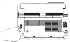
2. Insert the other end of the telephone cable into your wall telephone socket.
